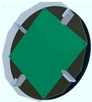
Before assembling, remove the protective film from the parts. Please note: when removing the film from the diffuser. This is transparent acrylic with tinting, do not remove the tint by mistake, only a protective film!
