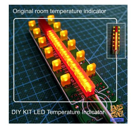
A set of parts for self-assembly of a digital indoor LED temperature indicator.
