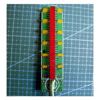
For the temperature indicator, select the red LEDs. For markers of tens of degrees of temperature - yellow LEDs.
